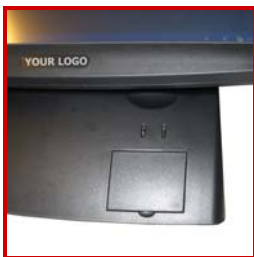
Hidden 2 USB ports and power switch. Status LEDs on front. Your logo/brand optionally.
