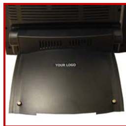
Rear cover hides cables connectors, but provides free tool access to I/O board and HDD.
